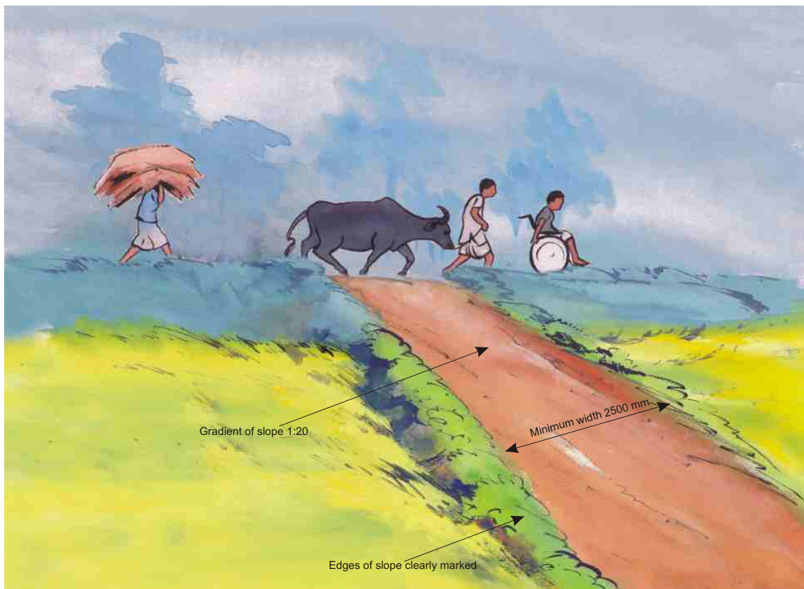
Straight slope to evacuation route
