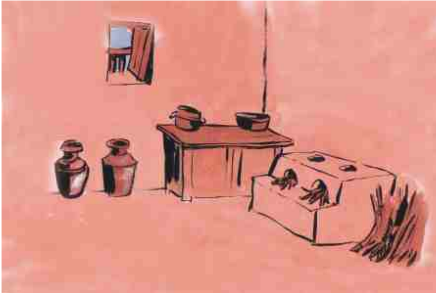
Raised mud-ovens can be ideal in an emergency shelter as long as a supply of wood is available
